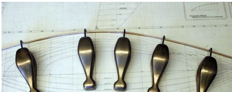
Figure 3: A physical drafting spline bent to model a smooth curve [15].
